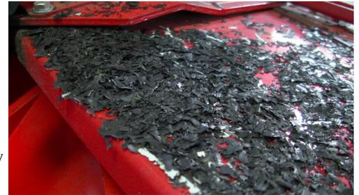
The newest service now offered at Gassman Automotive Products is Tire Truing! What is Tire truing you ask? Tire truing is the process of shaving thin amounts of rubber off of the high spots to transform an uneven tire into a round, even one. Having trued tires will enhance a rider's experience by creating a smoother, quieter ride, it will decrease uneven wear on tires, and will increase longevity of tires and associated steering and suspension components.
